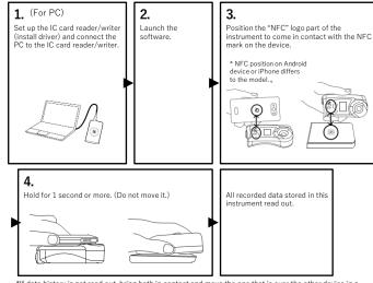
\*If data history is not read out, bring both in contact and move the one that is over the other device in a forward and back or left and right small motion.
